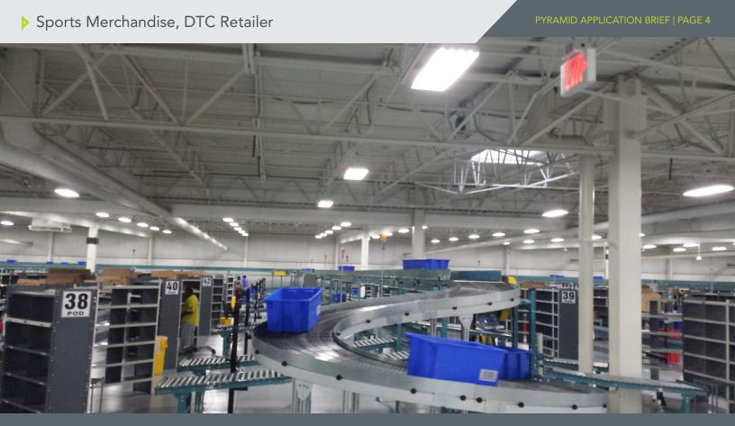
Pyramid Director WES and Case Sort Controller automatically route articles in totes picked by wave to an array of automated pack-out pods.
