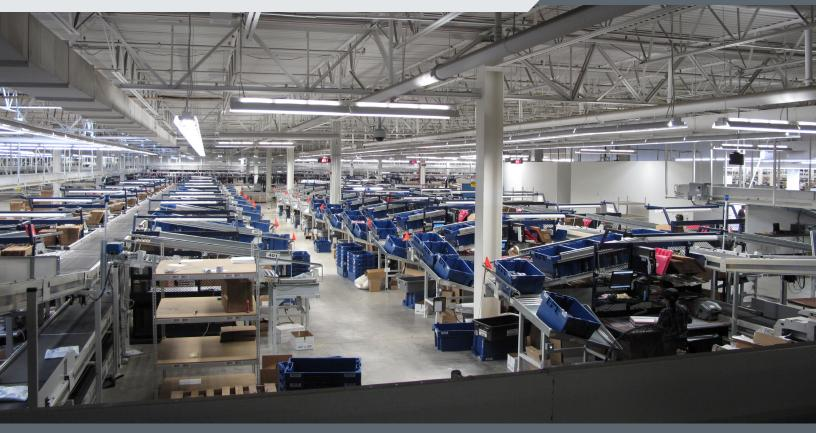
Pyramid Director WES routes customer orders to a network of 80 packing workstations, based upon packing attribute and workload balancing by workstation.
