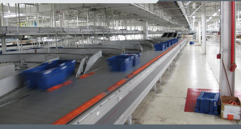
Totes of picked customer orders are routed across a high-speed slat sorter by Director WES for temporary storage or buffering into the packing sorter based upon critical flow optimization algorithms.
